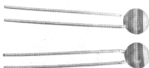
Resistencias NTC (Negative Temperature Coefficient).
